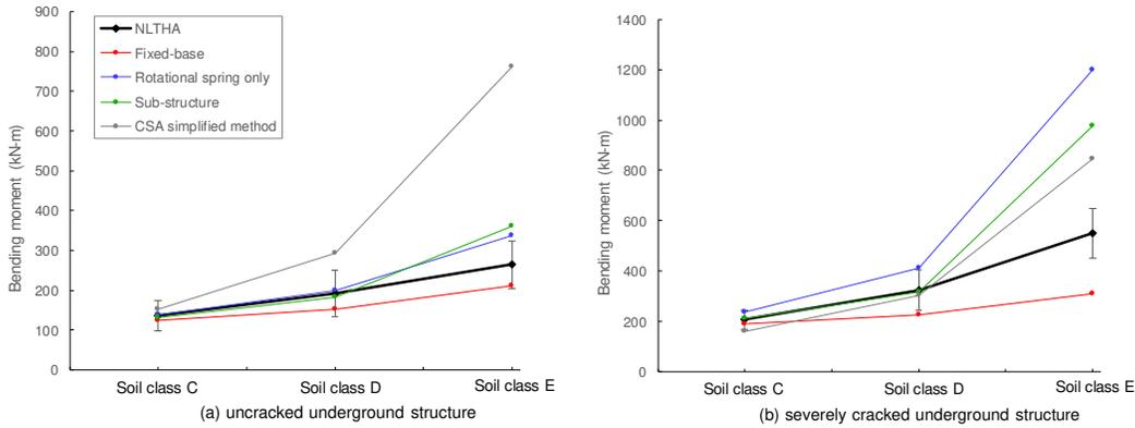
Figure 5. Elastic bending moment in the corner column at ground level. [Colour online].
