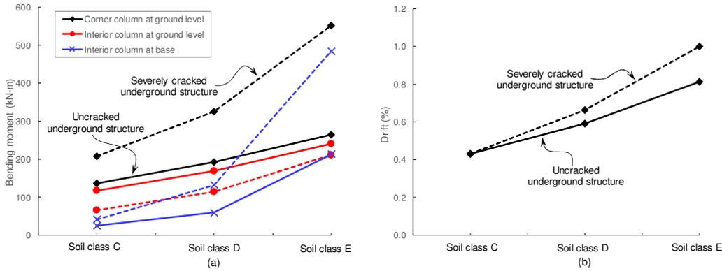
Figure 4. Results of NLTHA: (a) bending moment in columns, (b) drift at top of the building.
