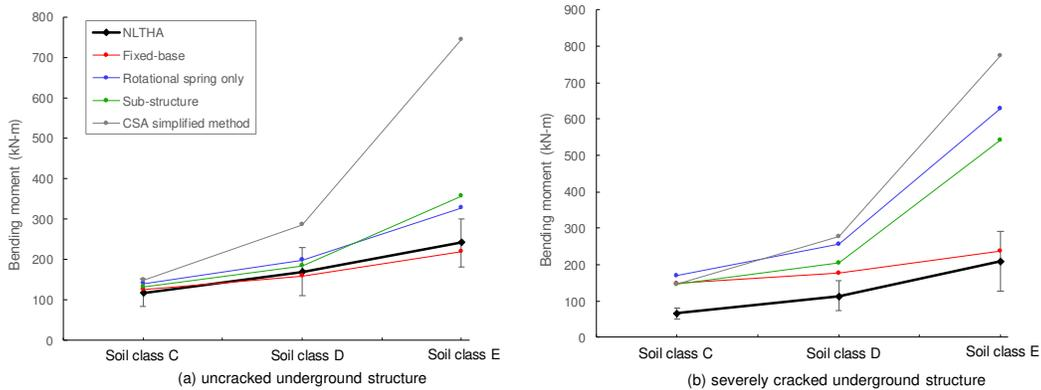
Figure 6. Elastic bending moment in the interior column at ground level. [Colour online].
