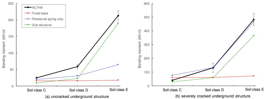
Figure 7. Elastic bending moment in the interior column at the base. [Colour online].
